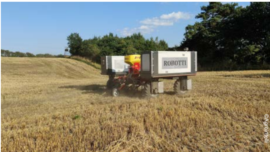
Figure 7. Self-powered platform (Agrointelli, Denmark)
