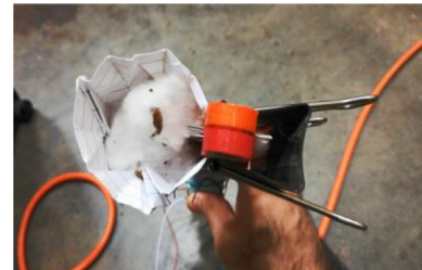
Fig. 4. The picked seed cotton got stuck while transferring to the doffing area.
