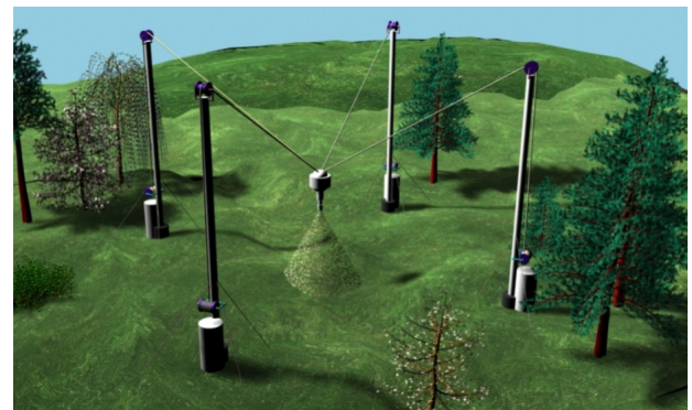
Fig. 1. A possible wire-robot structure for applications in agriculture.
