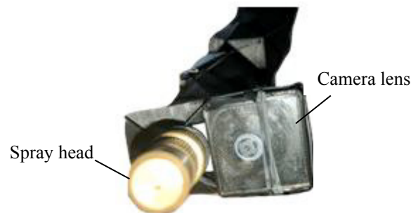
Fig. 7. Pi camera at the top of the arm.
