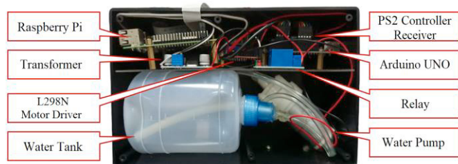
Fig. 9. Configuration of bionic arm control platform.
