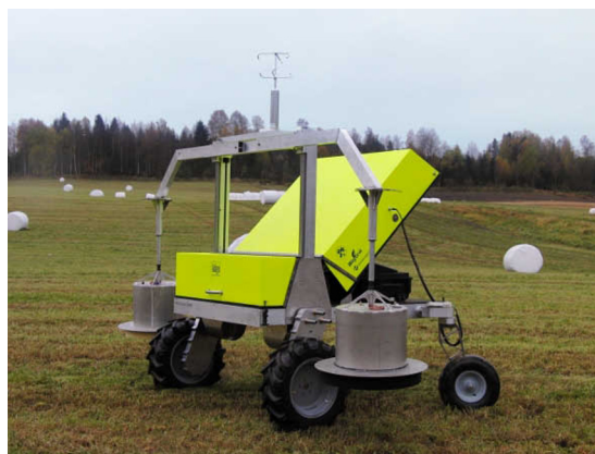
Fig. 1. A robot developed for autonomous N 2 O measurements on cereal fields. The robots autonomy is currently under development where efficient attitude estimation is a focus.
