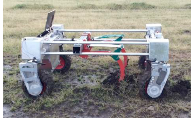
Fig. 7. Testing of robotic tillage in wet conditions during development of the initial Thorvald II prototype
