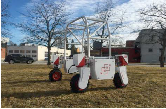
Fig. 5. A Thorvald II robot for cereal phenotyping. The high transverse arc allows it to drive over fully grown crops without damaging the plants.
