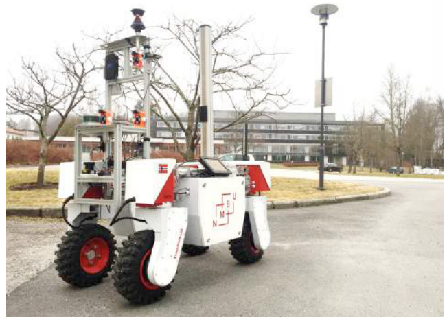
Fig. 4. Narrow Thorvald II robot for use in strawberry tunnels. The sensor mounting module prototype is clamped to the front of the robot.
