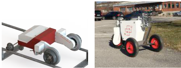
(a) A Robot for use in greenhouses (b) A three-wheeled Thorvald II robot during development
