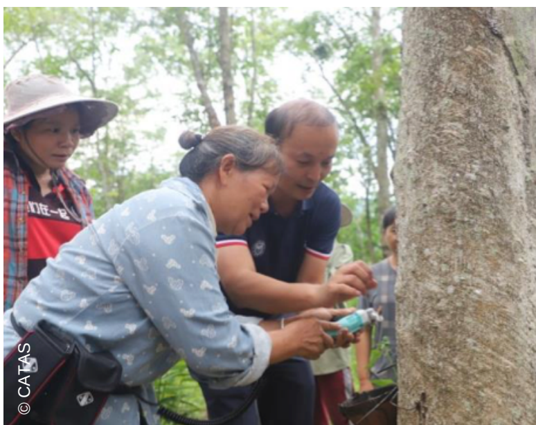
CATAS expert teaches farmers to operate the cordless electric tapping knife
