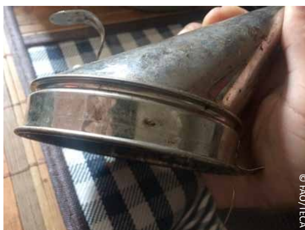
Figure 6: Coupling ring and a conical lid fixed
