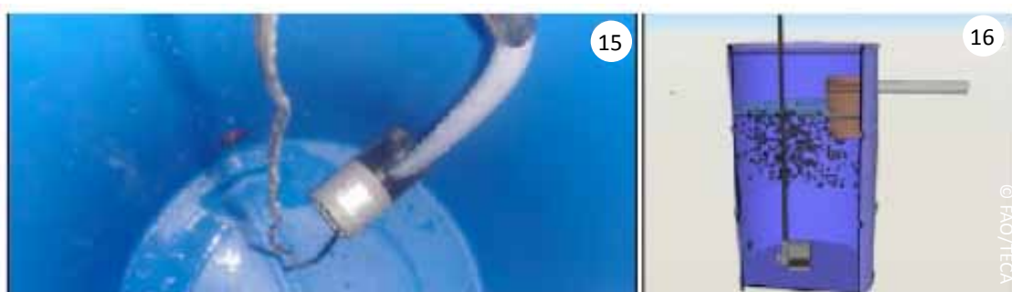
Figure 8: the Submersible pump is placed at the bottom of the biofilter barrel
