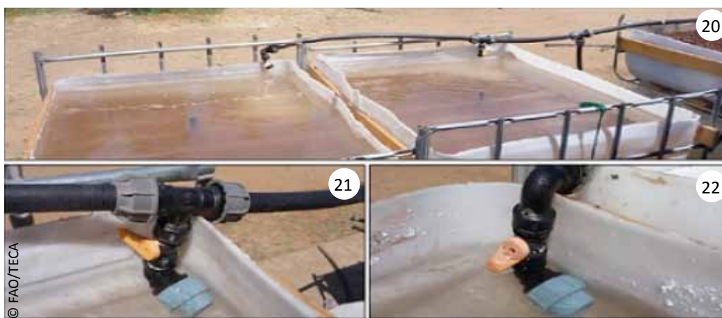
Figure 12: Connect the pipes to the metal frame with plastic cable ties
