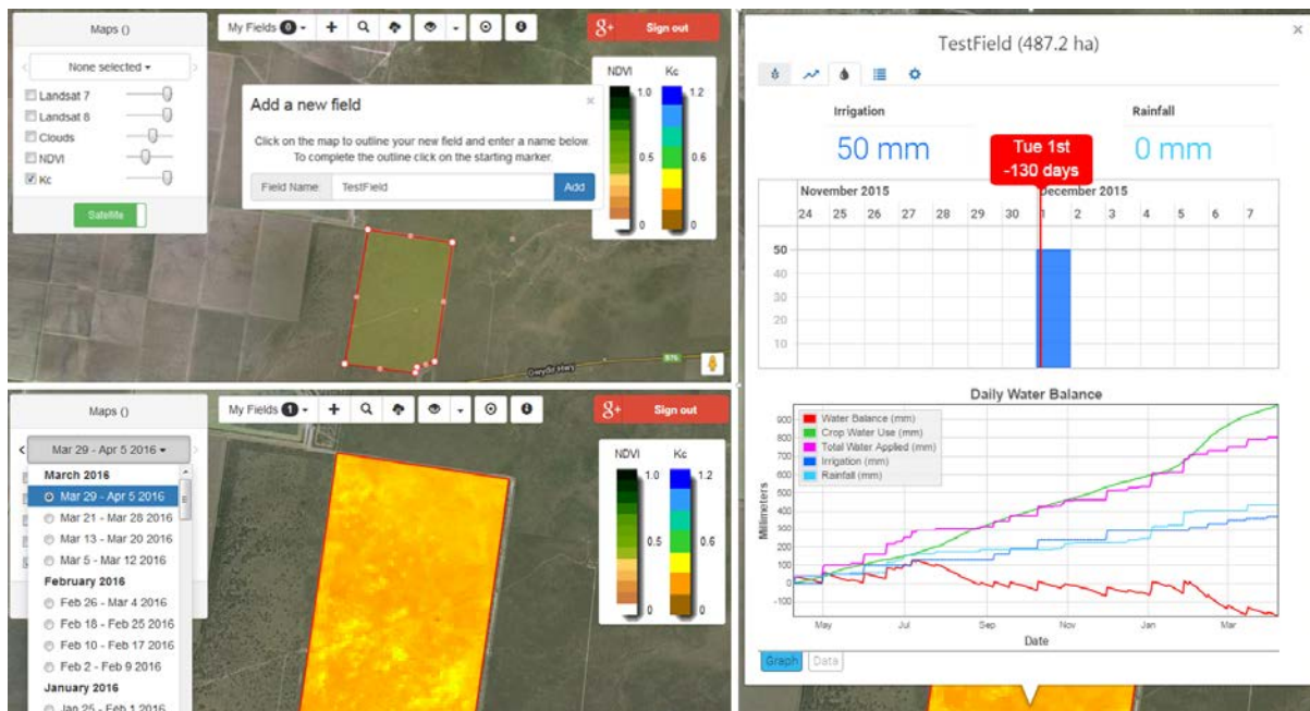
Figure 3: Three parts of the IrriSat web UI. Clockwise from top left: a user's new test field marked out ready for analysis; the waterbalance graph of the test field; the test field's crop coefficient taken from blended satellite imagery (LANDSATs 7 & 8)
